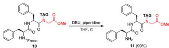
Scheme 4. Basic Deprotection of the Hydrophobically Tagged Tripeptide ( 10 )
